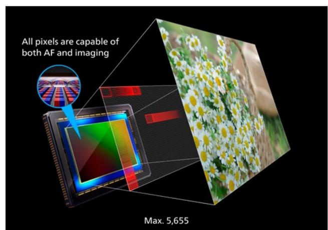
With the dual-pixel CMOS sensor, almost every pixel can provide both image and AF information.
