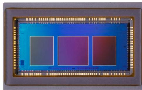
In DSLR cameras, a separate AF sensor is responsible for capturing the focus information, here the AF CMOS sensor from the EOS-1D X Mark III.
