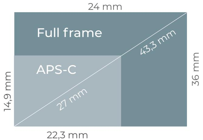
Size comparison: The surface area of the full-frame sensor is more than twice as large as that of the APS-C sensor.
