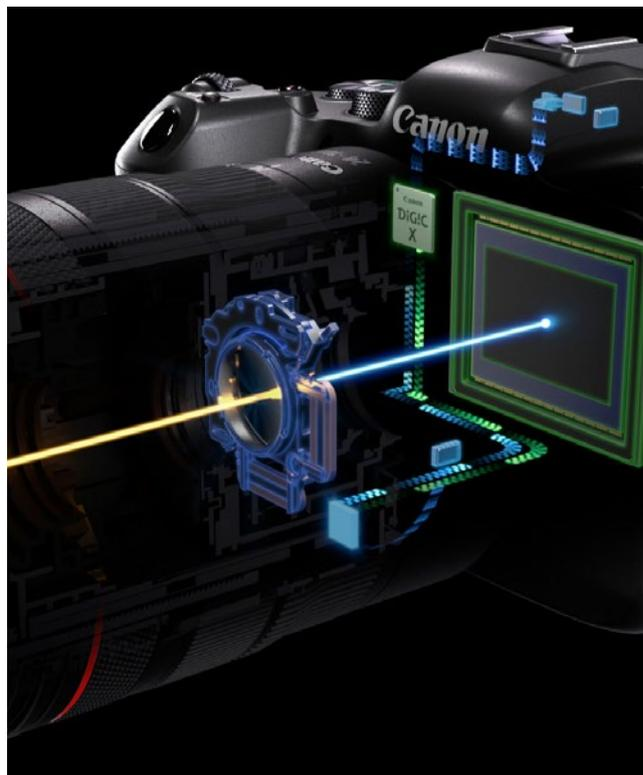
IBIS image stabilisation on the EOS R image sensor (green), combined with the image stabilisation of Canon's RF lenses (blue), allows you to shoot up to 8 stops longer without blurring caused by camera shake.
