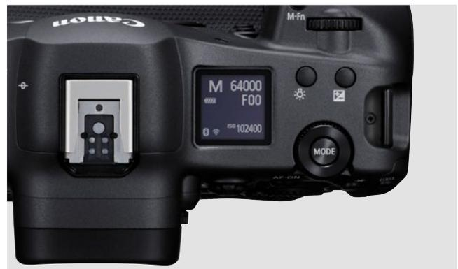
EOS R3: The high sensitivity of up to ISO 102,400 and the back-illuminated stacked sensor allow short exposure times, here 1/64,000s, with the electronic shutter.
